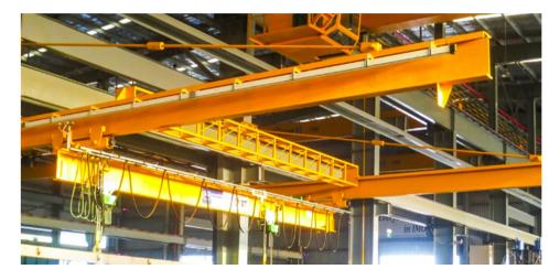
Single Girder Underslung Crane travels on the bottom of the runway girder beams mounted on ceiling of the building rather than building columns.
